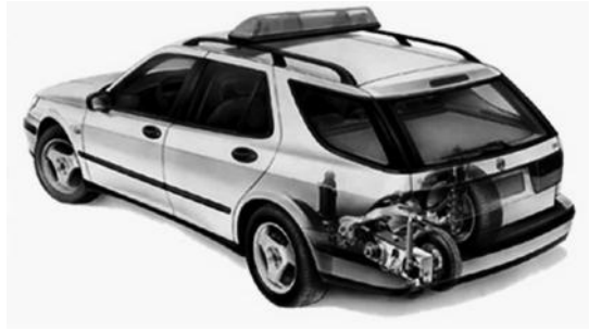
Figure 16.11 Sarsys SFT device. (Courtesy of Sarsys AB.)
