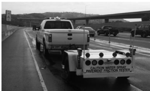
Figure 16.15 ASTM locked wheel skid tester. (Courtesy of Dynatest International A/S.)
