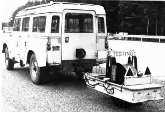
Figure 16.26 TRRL bump integrator on a trailer. (From Jordan, P.G. and Young, J.C., Developments in the Calibration and Use of the Bump-Integrator for Ride Assessment . TRRL Supplementary Report, SR 604. Crowthorne, Berkshire, UK: Transport Research Laboratory, 1980.)
