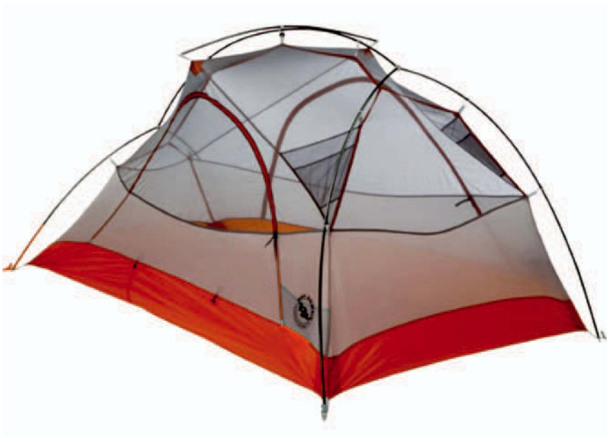
Figure 5.20 Copper Spur UL2 Tent. The backpacker's tent is an example of a short-span building for which the use of a highly sophisticated form-active structure is justified due to the need for minimal weight and therefore high structural efficiency. In this case the membrane is supported on compressive elements which are also form-active. A highly sophisticated structure of this type would not be justified for a building of this scale in which saving of weight was not critical.
