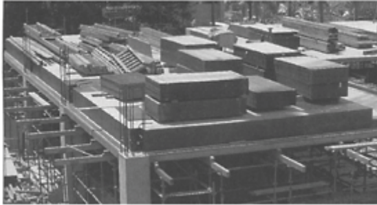
Example of Stage 1 Loading
